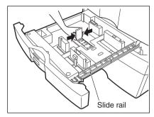
Push the arrow part (right side) of the size selection lever to unlock it.
